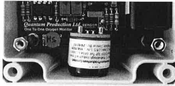
Figure 5-3 O2 SENSOR FITTED TO PCB
